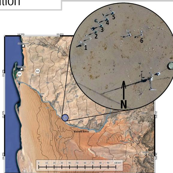
Figure 1: Overview map of the Central Namib, and location of the Gobabeb Namib Research Institute (GB). Upper right circle shows the measurement station in GB (birdview): 1: Harp, 2+5: Grunow-type, 3+4: Juvik-type fog collectors, 6: Thies Laser Precipitation Monitor
