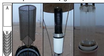
Figure 2: Grunow-type, Juvik-type, harp (from left to right), A: schematic drawing of the surface, which is incorporated in the calculation for the projected areas (whole area is considered), B: schematic drawing of impermeable material which is incorporated in the calculation for the initial interception areas (only solid fraction is considered)
