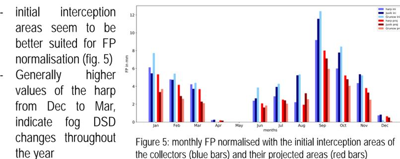
Figure 5: monthly FP normalised with the initial interception areas of the collectors (blue bars) and their projected areas (red bars)
