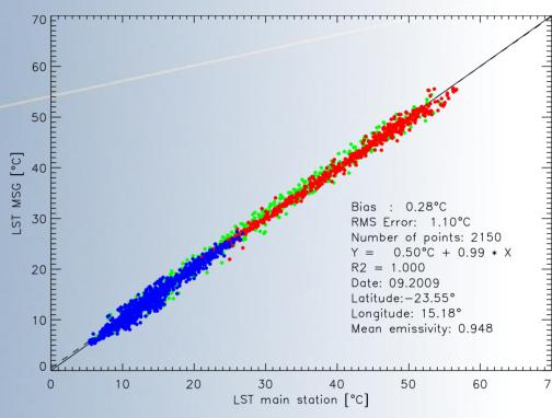
The plot shows LST obtained for the MSG satellite vs. Gobabeb main station LST for September 2009 (2150 valid data pairs). Colors relate to morning, afternoon and night. The data were matched to within one minute: the small bias & RMSE demonstrate the excellent quality of the satellite LST product.
