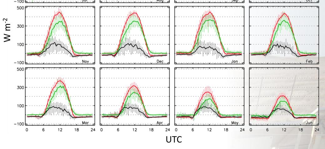
Mean monthly diurnal courses of the surface energy balance components. **Red** = available energy ( $Q^*+Q_G$ ). Green = sensible heat flux ( $Q_H$ ). Black = residual term. Until March 2011 latent heat flux was not measured directly and was assumed to be negligible.
