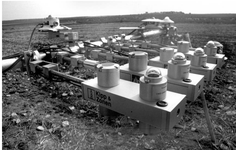
Fig. 2: Field calibration of the BUBBLE instruments in Southern Italy (“Bari 02”)
