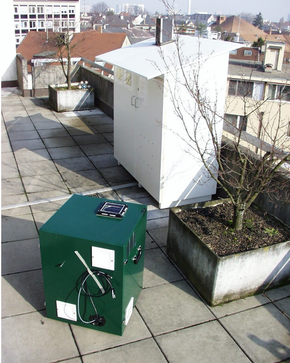
Fig. 1. View of the lidar on the 5 th floor balcony of the Institute of Meteorology, Climatology and Remote Sensing in Basel. The lidar itself is in the green box (protection and transportation). For long-term operation the lidar was installed in the white cabinet.
